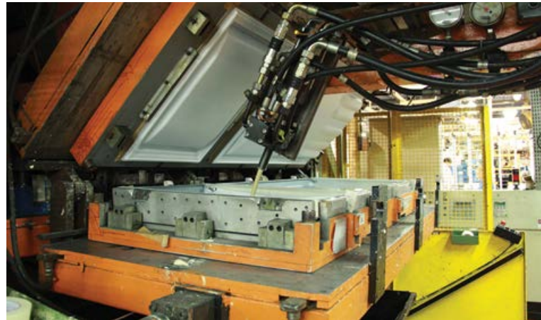
Refrigerator foaming process
